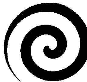
FIG. 2. In clockwise rotation, particles will be pushed away from the center of the spiral. In counterclockwise rotation, particles will be “collected,” or pulled in, by all points on the leading edge of the spiral.
