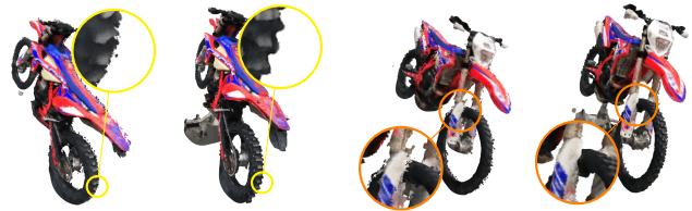
Figure 7. 3D Reconstruction from point clouds: The right object in each pair was reconstructed from DDNeRF, the left object was reconstructed from Mip-NeRF. DDNeRF achieves finer and less noisy shapes, especially around complex geometry regions.
