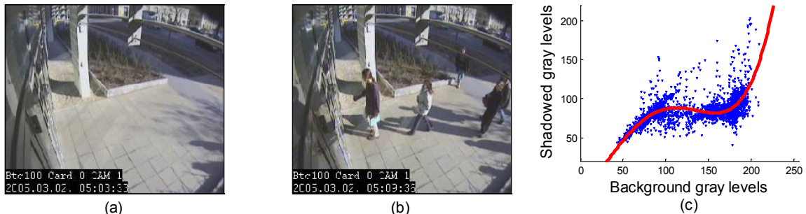
Fig. 1: Example of tone mapping due to shadows. (a) Background image of the sequence Sepm , (b) Frame #208 of the sequence, (c) The tone mapping applied to shadowed pixels of (b) is nonlinear.
