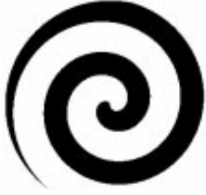
Figure 2: In clockwise rotation, particles will be pushed away from the center of the spiral. In counter-clockwise rotation, particles will be “collected”, or pulled in, by all points on the leading edge of the spiral.
